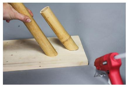
Make some holes with a drill making the 90-degree angle to the bamboo for the wood sticks, and with adding a little bit of wood glue insert the sticks. Create another level of the wood stick parallel to the bamboo. From the side, it will look like a grid.
